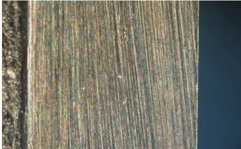
Base edge with SnowGlide machine with B25 stone (fine)
